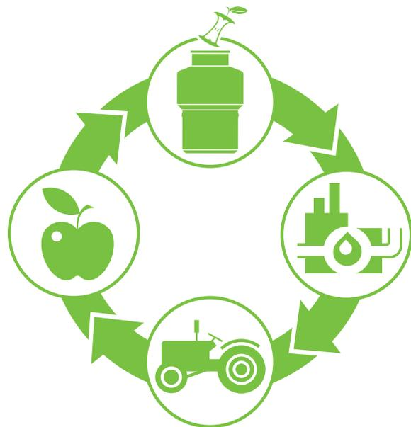
*This diagram shows how food waste disposers fit into the environment. First, food and food scraps are put through a food waste disposer. At waste facilities, biosolids are then captured and turned into fertilizer; methane gas produced during treatment is captured and recycled to power the plant or other facilities. Finally, biosolid fertilizer is beneficially applied to agricultural land that produces food, and the cycle begins again.*
